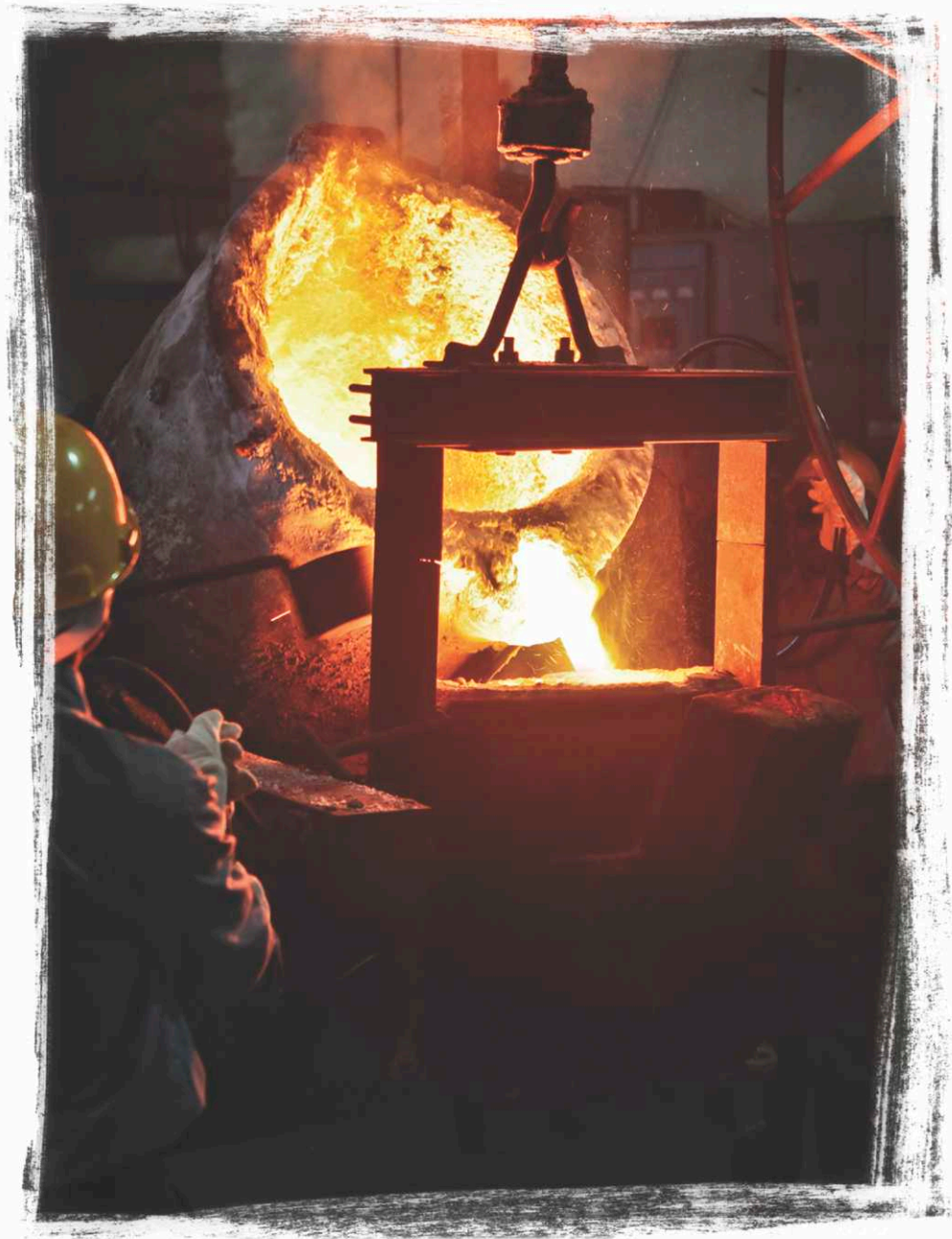
Ferrous Casting Dual Track Furnace
